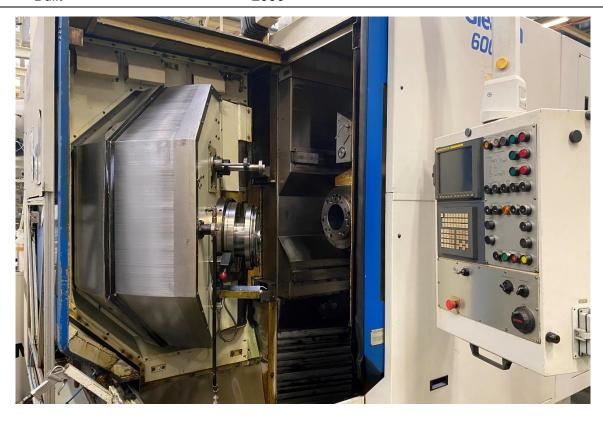
With the GLEASON Phoenix® 600HG bevel gear grinding machine, manufacturers of medium-sized spiral and hypoid bevel gears can achieve faster grinding cycles and higher accuracies at lower grinding costs.
